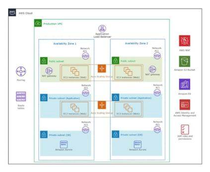
The architecture diagram shows how "AWS" cloud architect is powered by distributed servers and database services across multiple zones to ensure disaster recovery on deployment across multiple data centers, once the Application Load Balancer (ALB) detects the primary unavailable then it will direct all traffic to other in-service data centers.<sup>29</sup>
